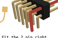
Fit the 2 pin right angle header for the FTDI 5v Input with the pins pointing to the outside of the board. Fitting a jumper to this before soldering will help keep it level.
